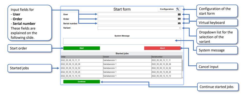
The design of the assembly order number, the serial number and the variant can be chosen freely (including special characters). In order to avoid incorrect entries, a filter for the input can be set in the configuration. This is explained in the Quickstep: **"0.3-QS\_Start form"**.
